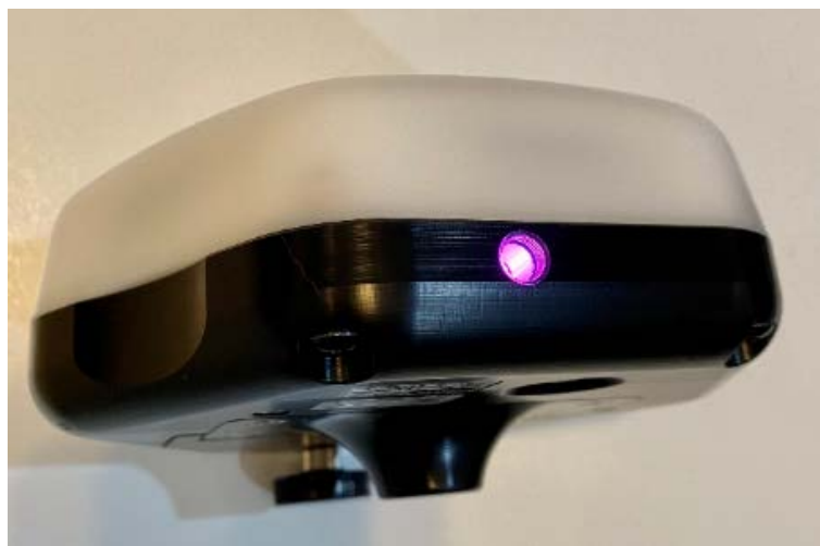
Figure 12. RTK Base Station Antenna with Indicator Light
