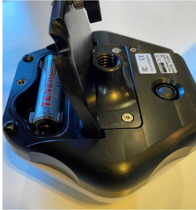
Figure 11. SonTek Base Station with Battery
